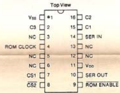
Pin Configuration for SPR016
