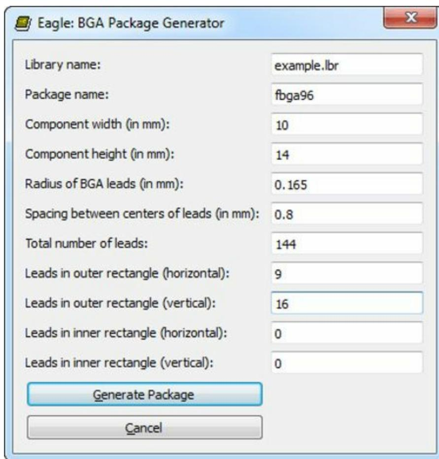
**Figure 15.5: The make\_bga\_package Dialog with MT41K Parameters**
